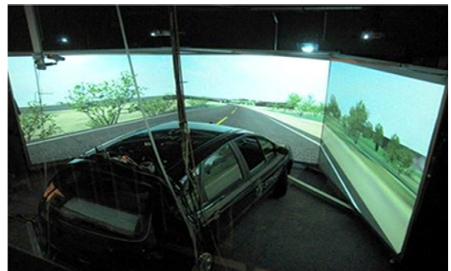
Fig. 3. Setup of the driving simulator. Vehicle and surrounding frontal screens.
