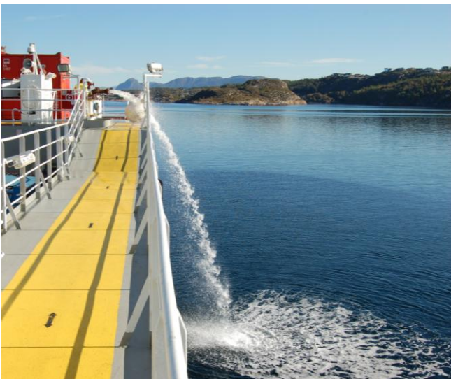
Figure 7.7: Dumping of potable water from tank. It is recommended to dump “old” water prior to bunkering. This applies to both supply vessels and offshore units (Photo: Eyvind Andersen)
