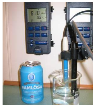
Figure 4.8: Some natural mineral water has very high sodium content, as the conductivity meter shows (Photo: Eyvind Andersen)
