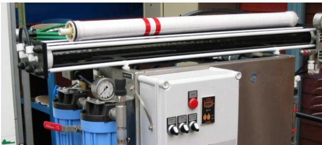
Figure 6.6: Reverse osmosis unit with the membrane placed in the roll on top of the unit (Photo: Bjørn Løfsgaard)
