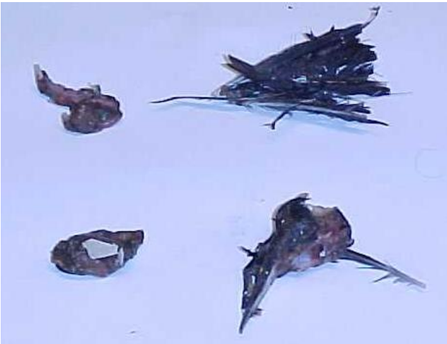
Figure 5.6: The remains of a bird collected from offshore potable water tanks. The bird entered via the bunkering hose, got stuck in a valve, and was spread to all the water tanks as it gradually decomposed (Photo: Anonymous in agreement with the company)
