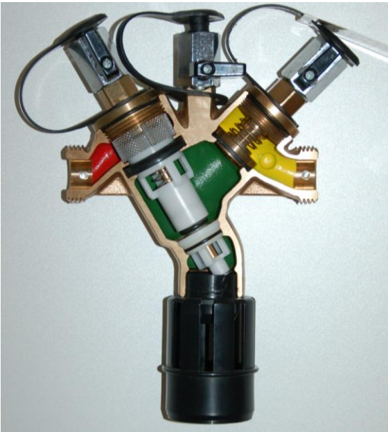
Figure 9.13: Other liquid carrying systems should not be connected to the potable water. If this can not be avoided a type BA backflow prevention device give the best level of protection. Note the 3 test points on top of valve. This valve needs to be fitted with a strainer and stop valves before and after for testing (Photo: Eyvind Andersen)
