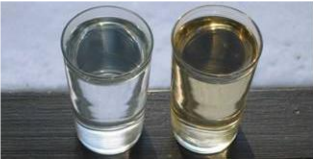
Figure 8.2: Water discoloured by humic material needs more chlorine than clear water to achieve a proper disinfection (Photo: Bjørn Løfsgaard)
