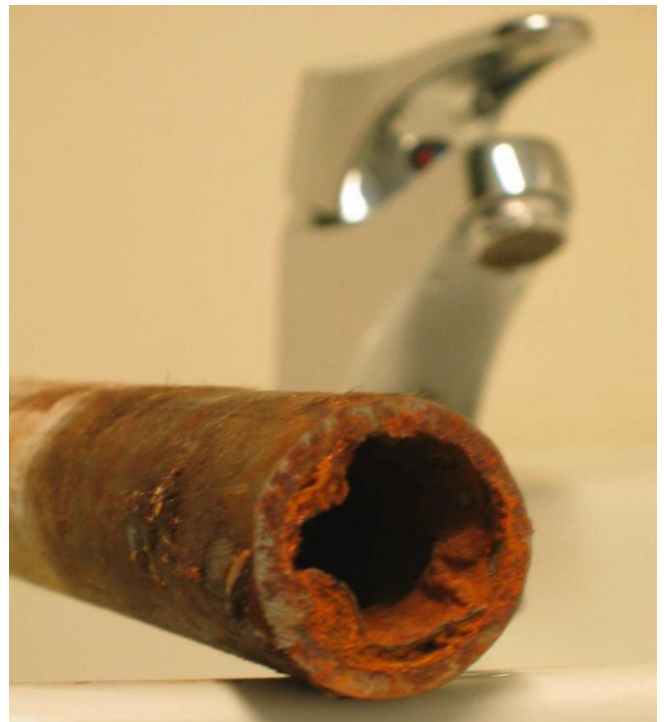
Figure 4.3: Corrosion clusters can result in poor water quality and clogging of pipes (Photo: Eyvind Andersen)
