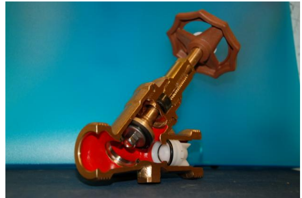
Figure 9.14: Verifiable non return valve with integrated stop valve. The test port is between the white non return valve and the screw down stop valve (Photo: Eyvind Andersen)
