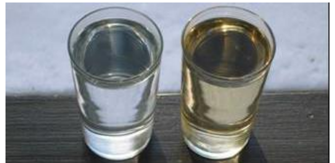
Figure 8.2: Water discoloured by humic material needs more chlorine than clear water to achieve a proper disinfection (Photo: Bjørn Løfsgaard)
