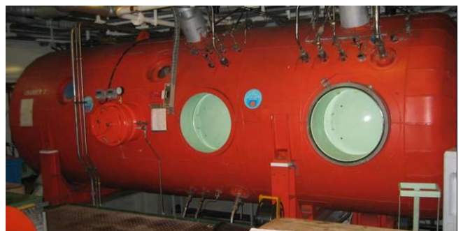
Figure 10.1: Pressure chamber designed for diving operations (Photo: Eyvind Andersen)
