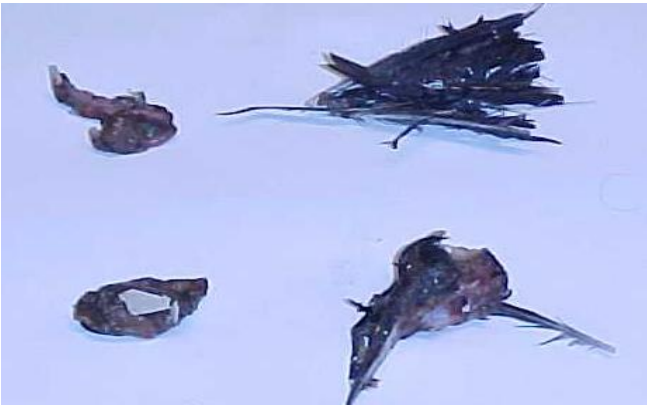
Figure 5.6: The remains of a bird collected from offshore potable water tanks. The bird entered via the bunkering hose, got stuck in a valve, and spread to all the water tanks as it gradually decomposed (Photo: Anonymous in agreement with the company)
