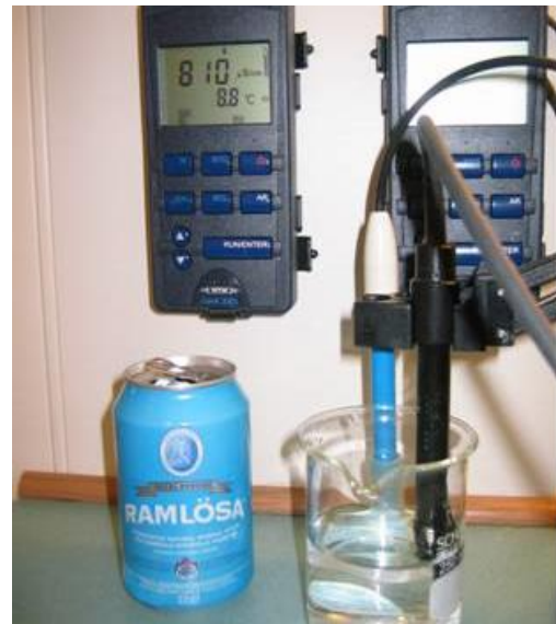
Figure 4.9: Some natural mineral water has very high sodium content, as shown by the conductivity meter (Photo: Eyvind Andersen)
