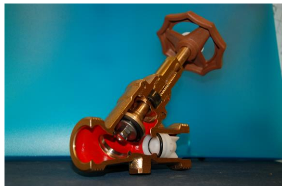
Figure 9.18: Verifiable non-return valve with integrated stop valve. The test port is between the white non-return valve and the screw down stop valve (Photo: Eyvind Andersen)
