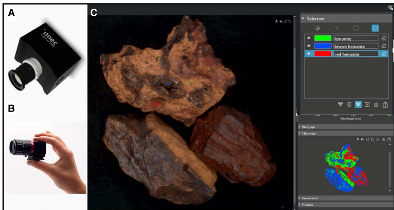
Figure 3. (A) imec Snapscan VNIR hyperspectral camera with LS150+ bands in 470–900nm. (B) Compact hyperspectral imaging (HSI) camera. (C) HSI image with robust classification of different ore oxide minerals with various colors and different chemical composition
