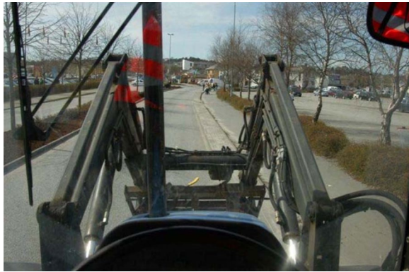
Fig. 7 The front end loader on tractors or similar vehicles also creates forward-looking blind spots, which have similar basic properties as those created by A-pillars. From Ringen and Moss-Iversen (2017), reprinted with permission
